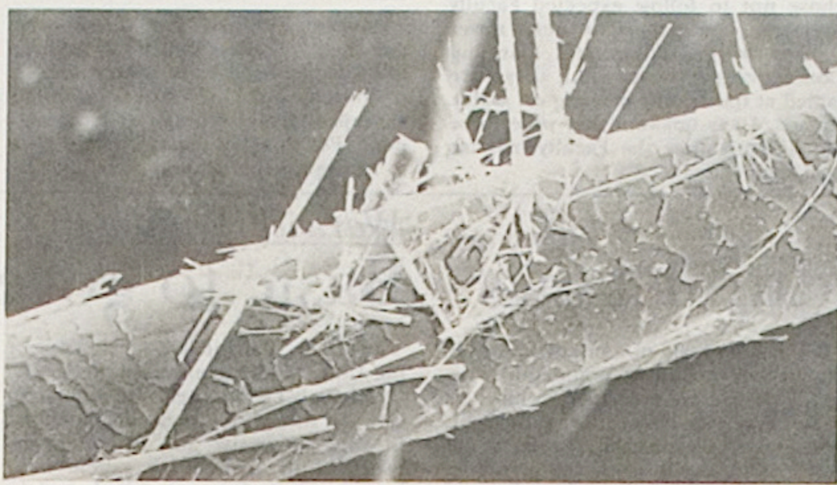
Asbestos fibres clinging to a strand of human hair seen through the scanning electron microscope and magnified 1300 times. Photo: Roger Heady and Nick Mackie.
