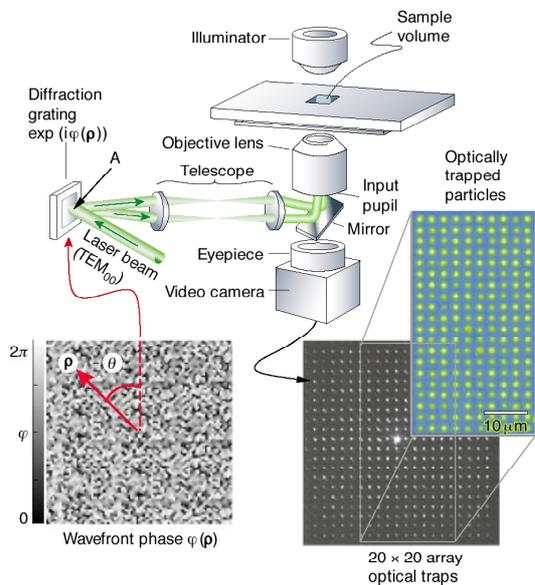
Figure 12: Schematic of an advanced OT set-up using holographic interference to create a dynamic array of traps. Using a computer-controlled Spatial Light Modulator (SLM) in place of the hologram, one can create optical vortices or rotator traps which impose twist-like torques on particles. The SLM also allows one to dynamically change the array dimensions. From Grier [4].
