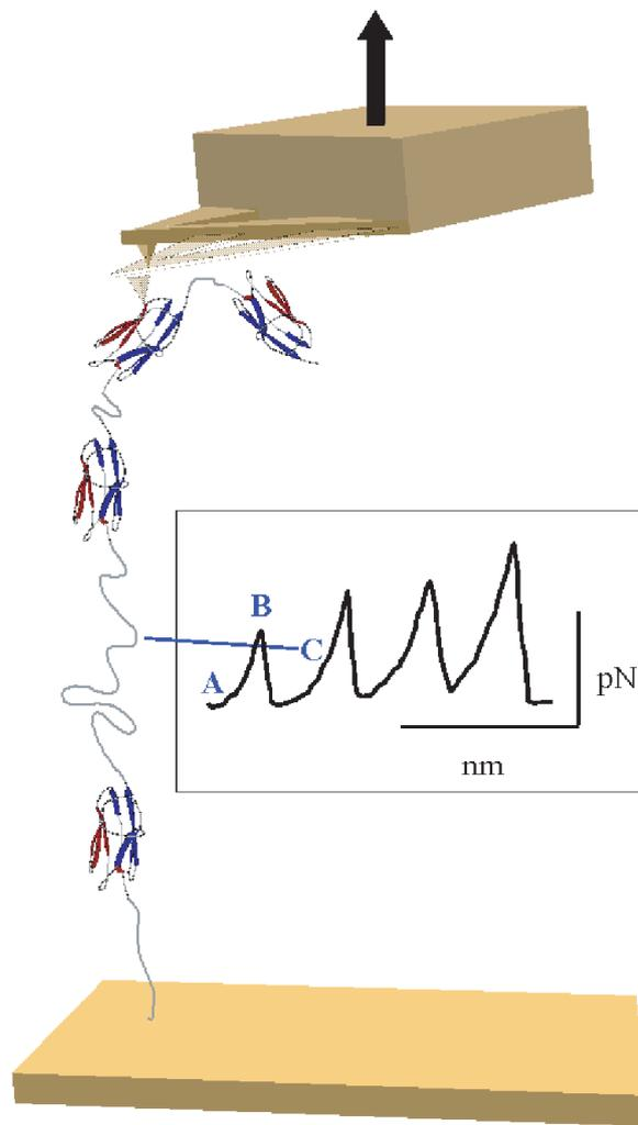
Figure 8: Schematic of AFM stretching a biomolecule, from <http://www.astbury.leeds.ac.uk>
