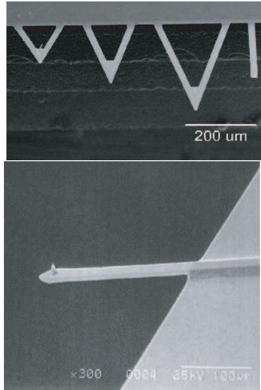
Figure 6: Electron micrographs of AFM cantilevers, from <http://www.astbury.leeds.ac.uk>
