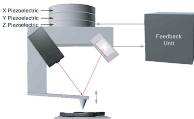
Figure 5: Schematic of an Atomic Force Microscope, from [http://www.pacificnano.com/afm-tutorial\\_afm-instrumentation.html](http://www.pacificnano.com/afm-tutorial_afm-instrumentation.html)
