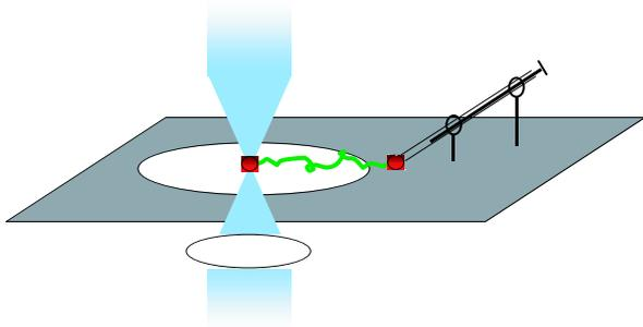
Figure 11: Schematic of how a DNA molecule is stretched in an OT apparatus
