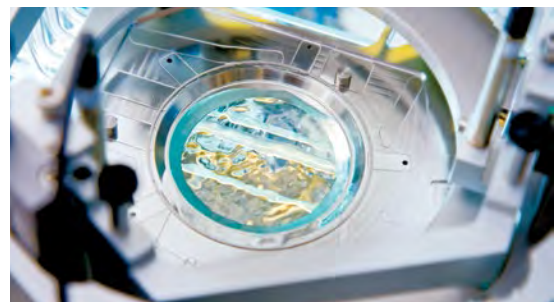
This immersion scanner, made by ASML, is used in multiple patterning, one of several advanced photolithography methods driving demand for semiconductor materials.
