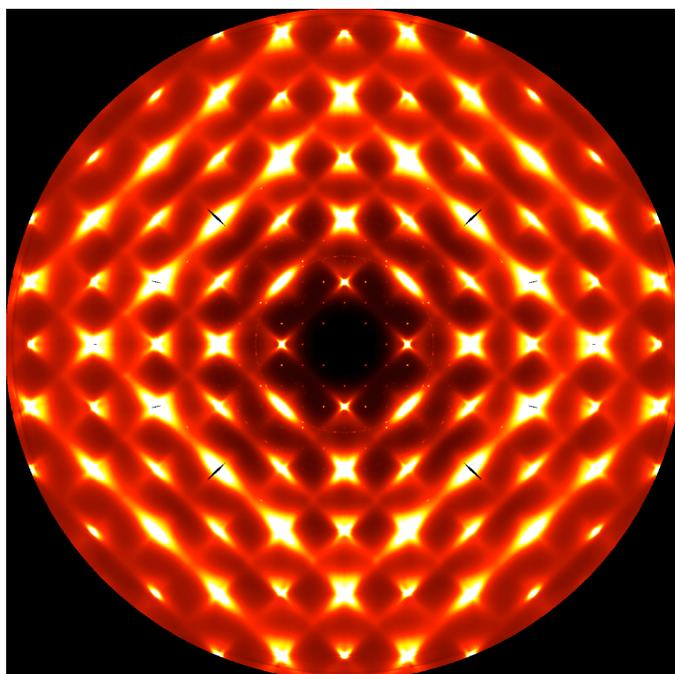
Figure 1: Diffuse X-ray scattering, measured at the Advanced Photon Source Synchrotron in Chicago. The material is PZN ( $\text{PbZn}_{1/3}\text{Nb}_{2/3}\text{O}_3$ ), a material with electrical properties that make it useful in fields like energy conversion and micro-actuators.
