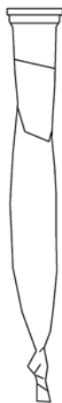
Fig. 1: Schematic drawing of the assembly of the cut Eppendorf tube in the knotted dialysis bag to provide a readily accessible container for the reaction mixture.
